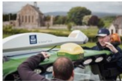
N-Sensor: A tractor-mounted vegetation sensor.
